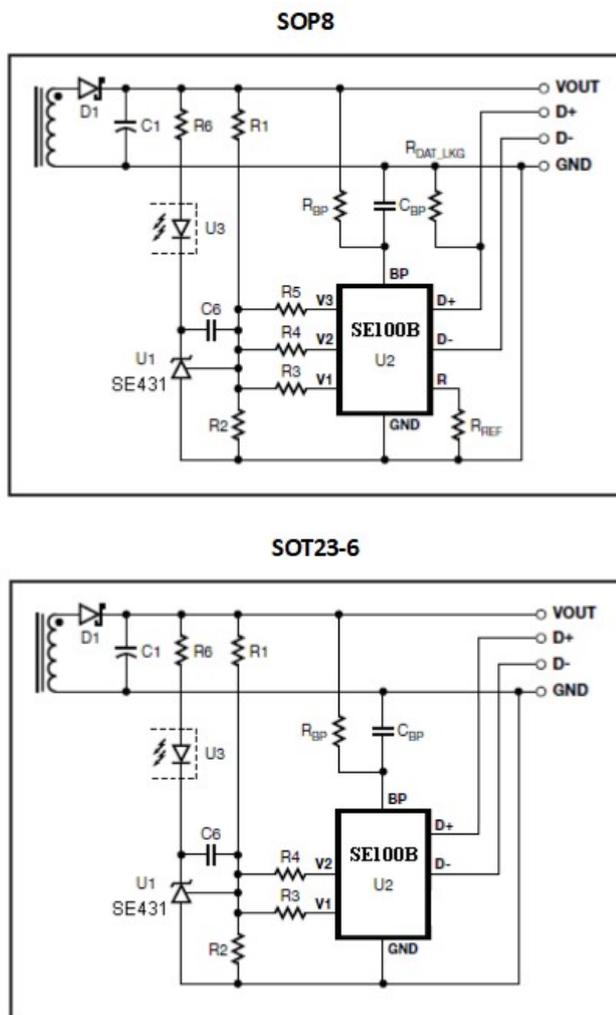
Figure 1. SE100B with Traditional Output Regulation (CV Only).
