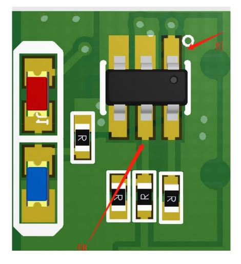
Please note that LED pin carries strong digital signal and FB pin is the high impedance pin. We intentionally separated these two pins on two sides of the package. It is important to continue placing the related PCB trances on both sides of the PCB so that the LED digital signal will not interfere with the FB pin during the LED transition period. If it is necessary to place them close to each other, please add a GND trace to provide a ground loop for better isolation.
